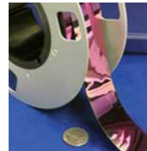
High temperature superconducting tape – courtesy American Superconductor®
