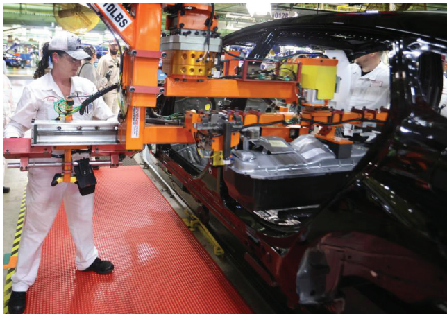
An associate at the Marysville Auto Plant installs a battery in a hybrid Accord.
